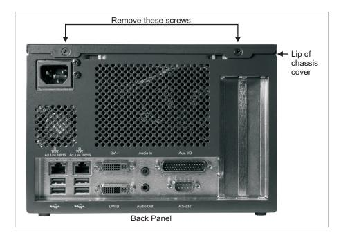
3. The back of the chassis cover has a lip that snaps on to the unit. Push up on the lip. Carefully open the cover all the way. You will notice that the hard drive is attached to the cover. Be careful not to pull on the hard drive cable.
