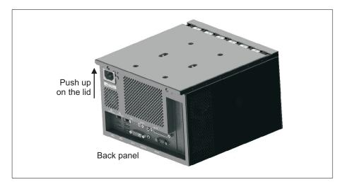
Use caution when inserting and removing components with the chassis cover open. The cover leans at an unstable angle and could fall.
