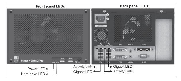
There are a total of six clearly-labelled LEDs on the Matrox 4Sight GP unit.
