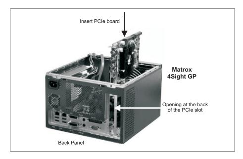
3. Press the board firmly but carefully straight down into the connector of the slot.
